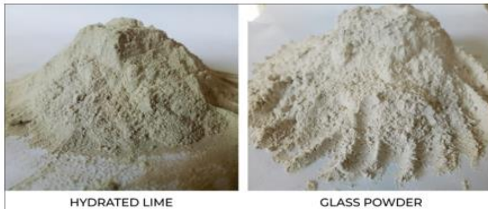
Figure 2: Hydrated Lime and Glass Powder used as Non-Conventional Fillers.
