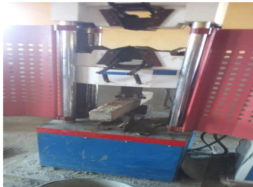
Fig. 3: Flexural strength test of round bamboo reinforcement beam
