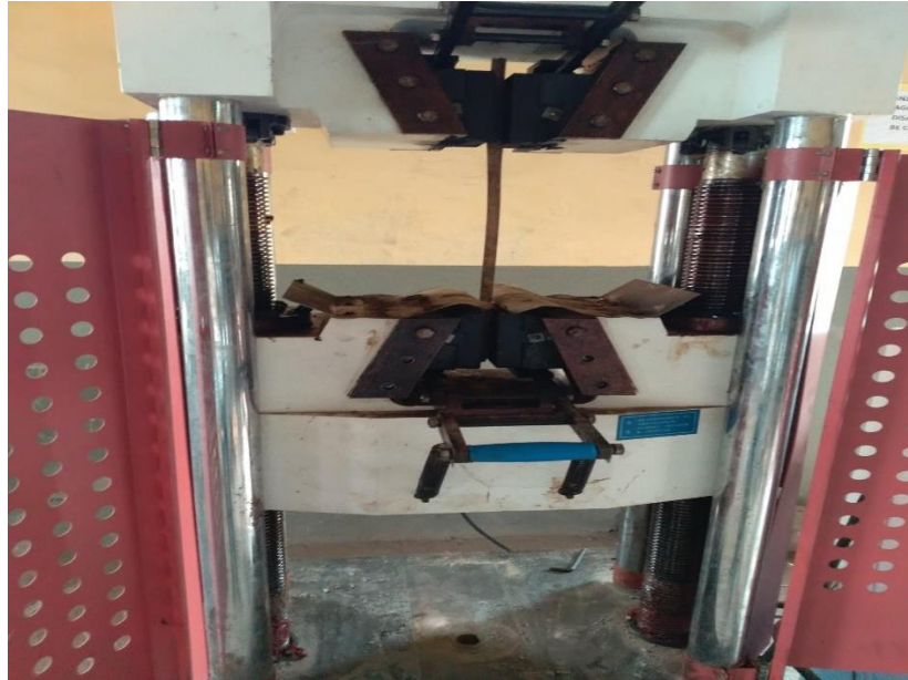
Fig. 2: Tensile testing of flat bamboo reinforcement
