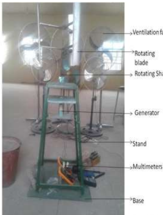
Plate 1: Experimental set up of Conventional VAWT
