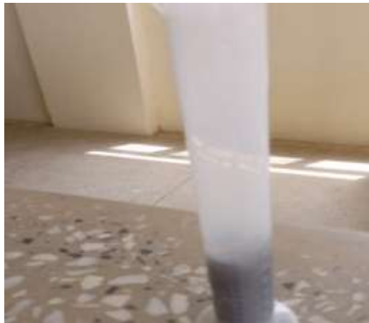
Plate 4: Set up for determining the volume of the sample through displacement method
