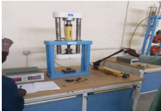
Plate 5: Testing of the Compressive Strength of Brachystegia eurycoma using UTM
